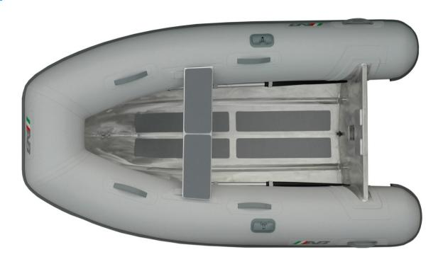
**Overal Length** : 9'1"/ 2.76m Number of Chambers : 2 Shaft Length : 15" / 38.1cm **Person Capacity Overal Beam** : 4'11"/ 1.50m RDC Design Category : C Inside Length : 6'3"/ 1.90m Weight : 75lb / 34kg Recommended HP Inside Beam : 2'3"/ 0.70m : 8hp / 6kw : 16"/ 0.41m Maximum HP **Tube Diameter** : 10hp / 7.5kw
